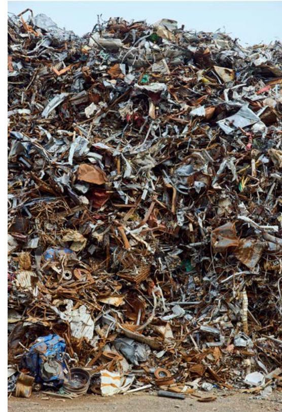
Scrap, ferro-alloys and other input materials contain carbon that needs to be removed from the steel to reach the specified chemical composition.
