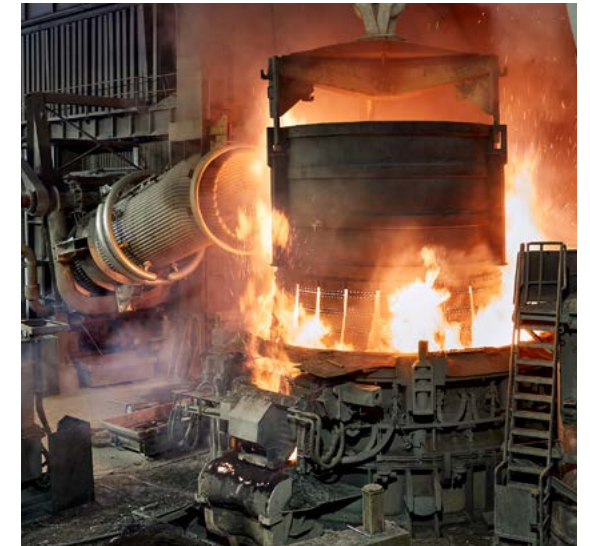
Swiss Steel Group produces exclusively from steel scrap. At the very beginning of the production process, the specially sorted scrap is transformed into liquid steel using electricity.
